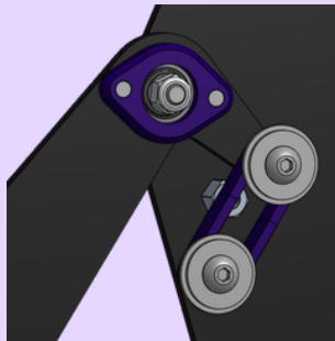
Passive rubber band extension to pivot out the pickup ramp plates
