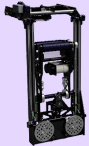
The full set of subsystems to handle catalysts, including the MGN differential lift, lightweight arm, and catalyst launcher
